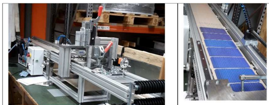
Figure 1: Semi-automated TECC-Wire solar cells stringing machine (left), and a full string of half-cut M6 HJT busbar-less solar cells
